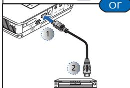
Connect the VGA / Component / HDMI device using an appropriate cable. (①~②)
