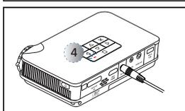
When the LED indicator lights red, the battery is low. Replace the battery immediately or connect the power adapter to charge the battery.
